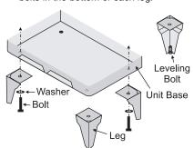
NOTE: Adding the legs changes the height of the unit, make sure you have sufficient clearance (min. 28") for your flue connection.
